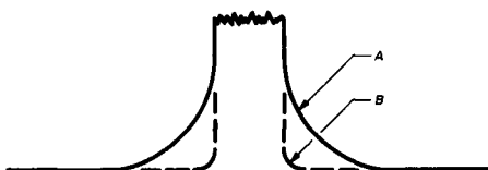
fig. 3. Display of filter response with noise generator input and SB620 installed after the filter. Curve B can be obtained with careful matching and tuning.
