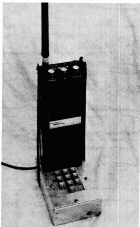
The Regency HRT-2 sits atop the charger overlooking the ever popular Touch-Tone pad.
